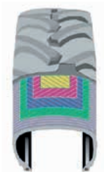
Radial tire construction: The cords are replaced towards the tire center with 90 degrees.
