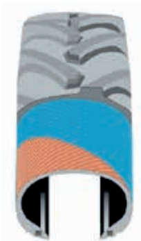
Bias tire construction: the cords are placed diagonally with certain degrees for the rotation direction of a tire.
